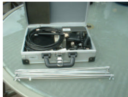
My travelling kit, FT817, charger cables, mic and ML-40 and ML-20
